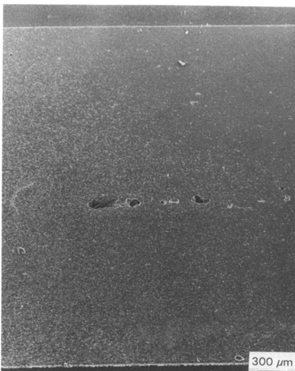
Figure 9 Fine pores seen at the centre of the cross-section of a sintered test bar.
